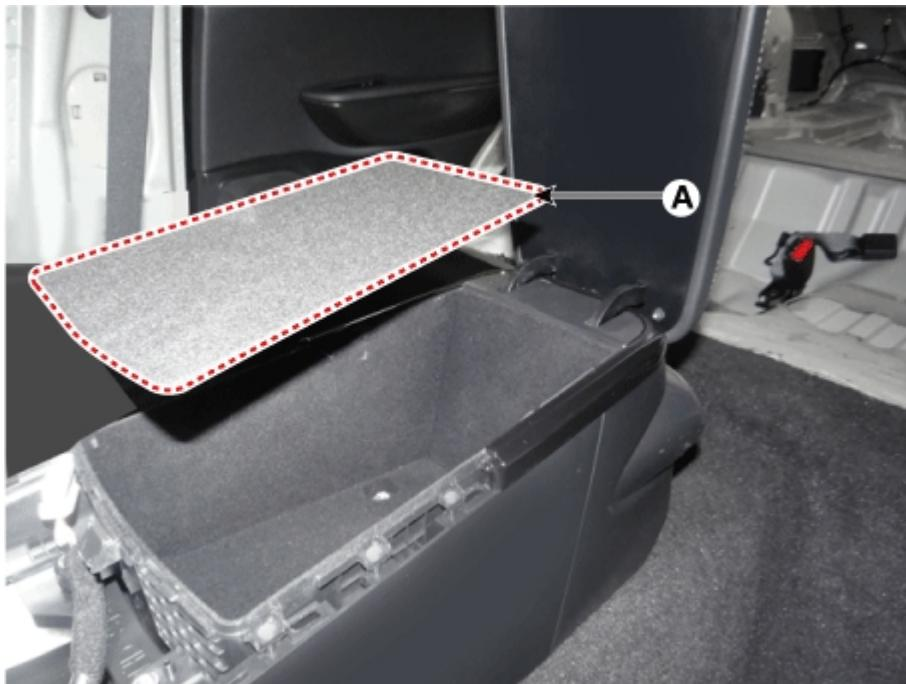
7. Remove the console side molding (A).
