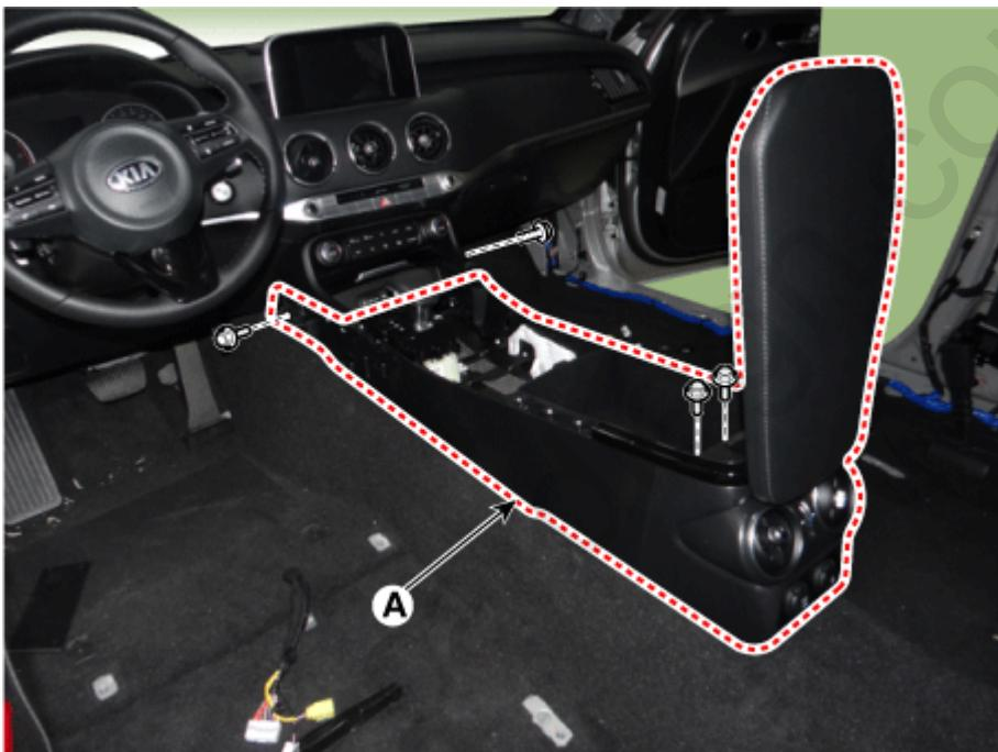
12. Remove the console front cover (A) after loosening the mounting screws.
