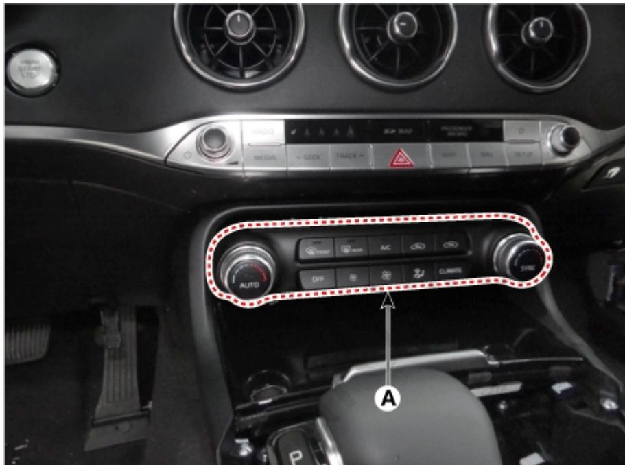
2. Remove the heater control unit after disconnecting the connector (A).
