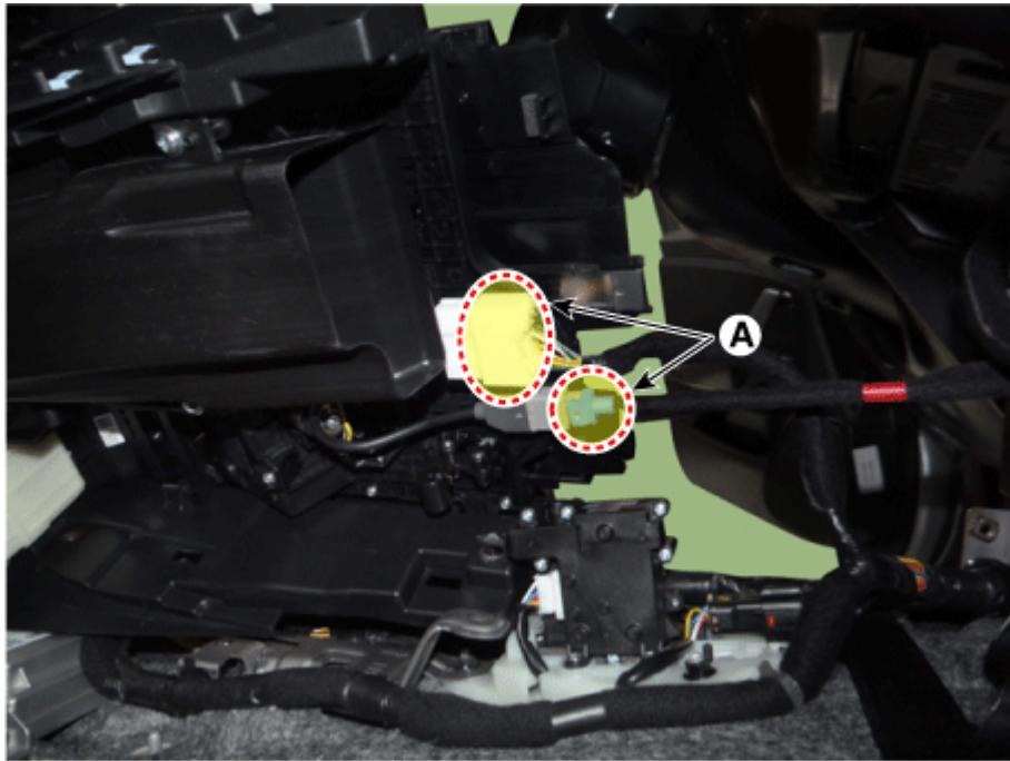
11. Remove the console assembly (A) after loosening the mounting bolts.
