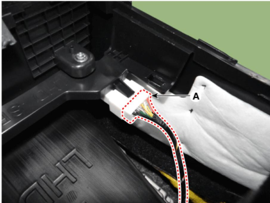
9. Disconnect the electronic shift lever connector (A).
