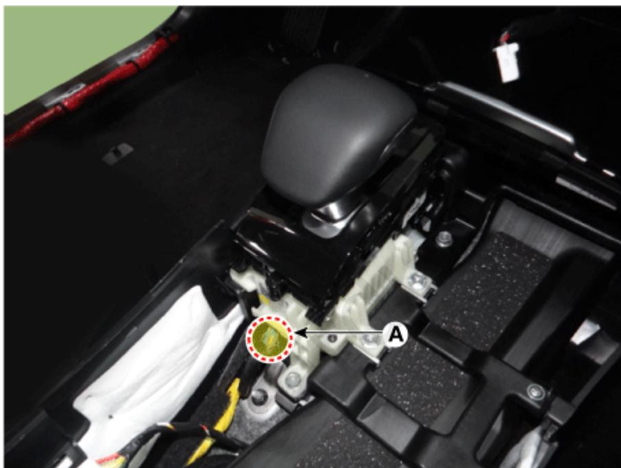
10. Disconnect the console lower side extension connectors (A).
