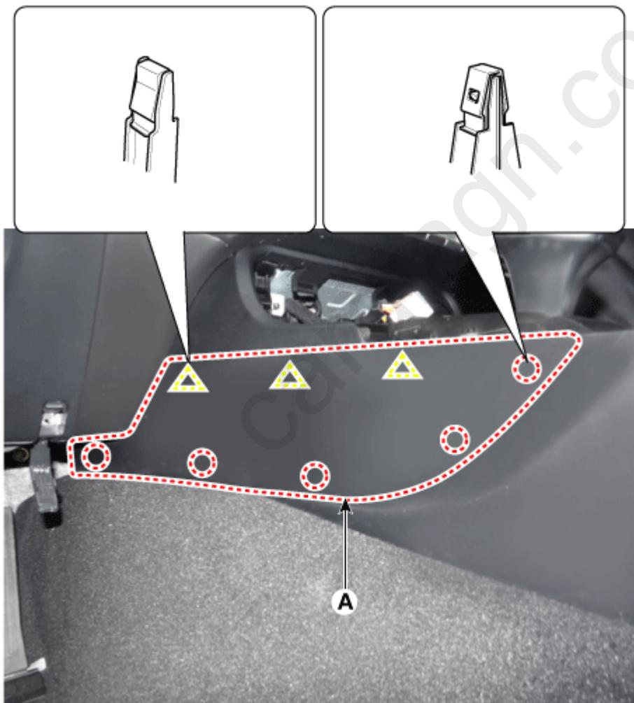
8. Disconnect the console upper side extension connectors (A).
