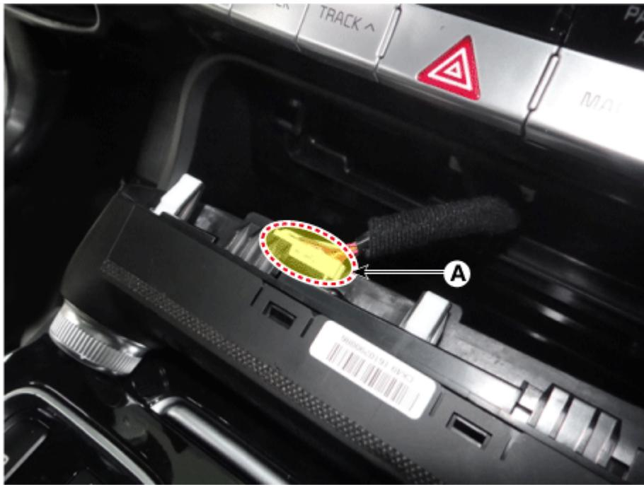
3. Remove the console upper cover (A) by using a remover.
